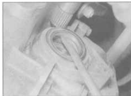
5.8 Levering a driveshaft and oil seal from the transmission
