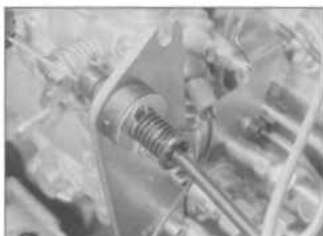
18.2 Accelerator cable adjustment ferrule on the Bosch injection pump
