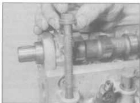
9.41A Cylinder head bolt with spiral grooving on its shank
