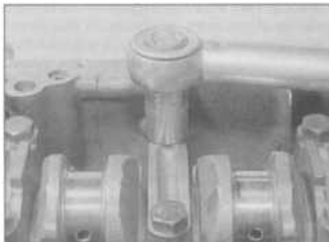
24.12 Tightening the main bearing bolts
