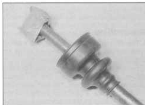
4.12 Inner rubber bellows located on the driveshaft
