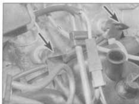
17.3 Plastic clips (arrowed) on heater plug terminals
