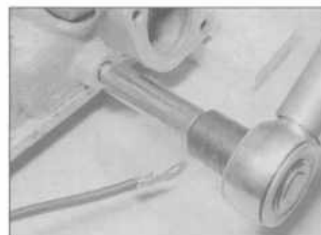
17.6 Tightening a heater plug
