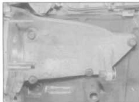
23.36 Injection pump mounting bracket
