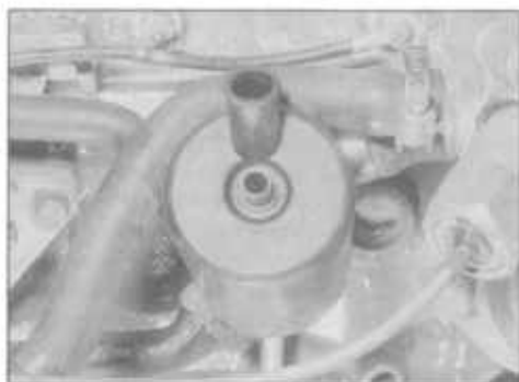
24.73 Oil separator located on the dipstick tube (1.9 engine)
