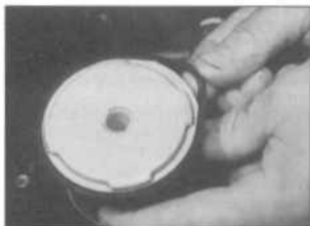
23.11D Checking the sealing rubber
