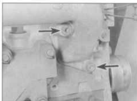
25.3A Inlet manifold bolts (arrowed)
