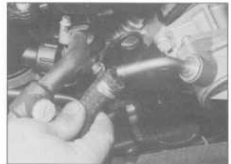
7.1 Disconnecting the vacuum hose from the vacuum pump
