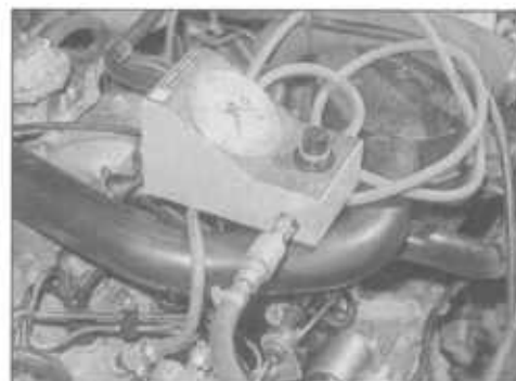
3.15 Leakdown tester in use
