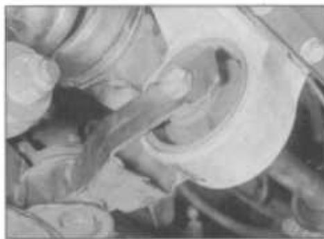
20.30 Engine lower mounting and torque link (BX models)
