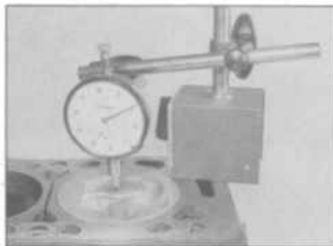
9.34 Checking the piston protrusion
