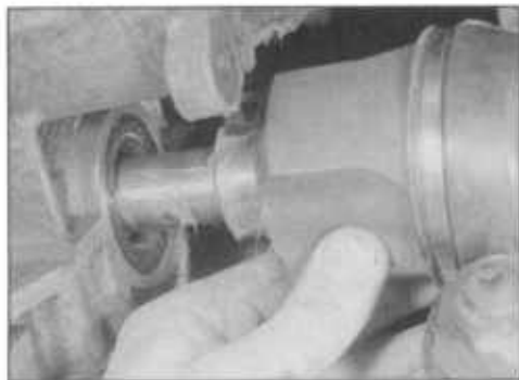
5.16 Refitting the left-hand driveshaft
