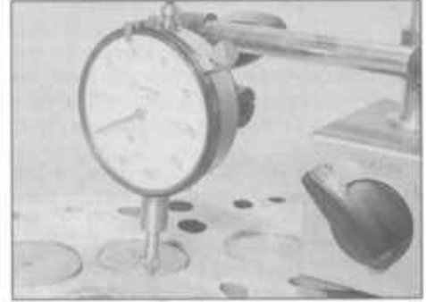
10.14 Checking the valve head height
