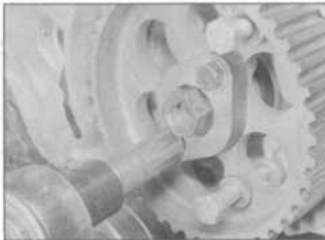
24.49 Tightening the special puller to the injection pump sprocket
