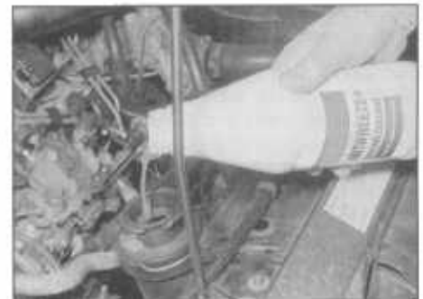
5.1 Filling the radiator on BX models
