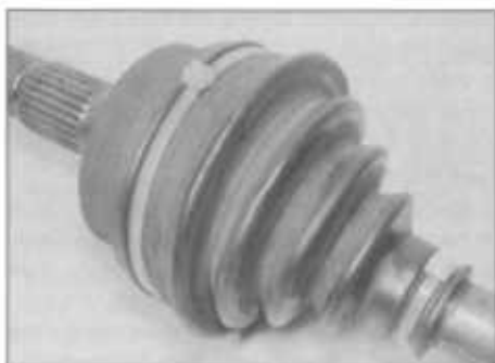
4.1 Plastic straps on the outer rubber bellows
