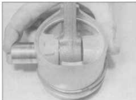
26.25B Pushing the gudgeon pin into the piston
