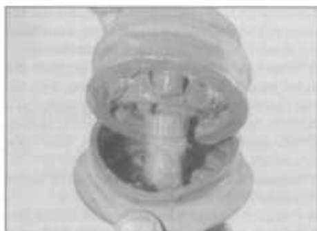
4.2 Removing the rubber bellows from the outer joint housing
