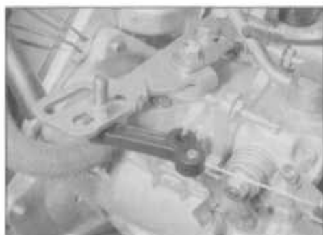
18.1B Accelerator cable attachment on the Bosch injection pump
