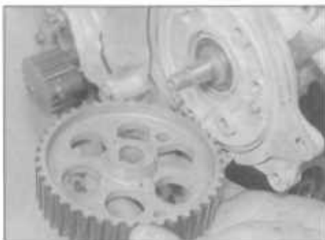
23.31B ... and remove the injection pump sprocket
