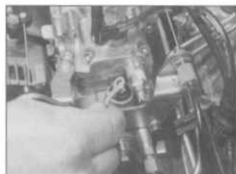
19.3 Disconnecting the wiring from the stop solenoid
