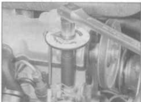
9.41C Angle-tightening a cylinder head bolt, using a commercially-available angle gauge
