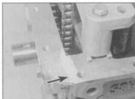
24.30A Apply sealing compound here . . .
