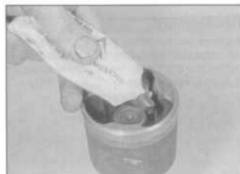
4.11 Injecting grease into the inner joint housing
