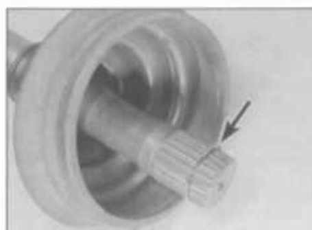
4.3 Driveshaft outer joint retaining circlip (arrowed)
