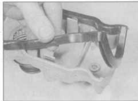
7.8B ... and remove the gasket
