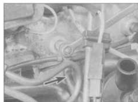
17.4B Removing the heater plug main supply cable (arrowed)
