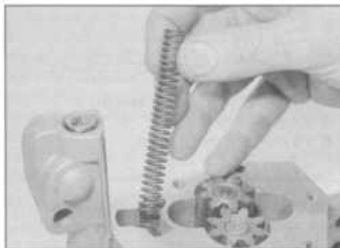
14.9C ... and remove the relief valve spring ...
