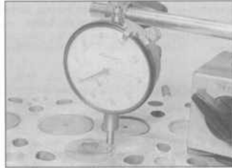
10.11B ... then check the swirl chamber protrusion
