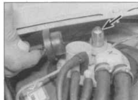
12.4 Filler cap removal from the hydraulic fluid reservoir Fluid level indicator location is arrowed
