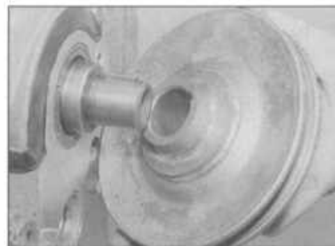
23.5 Removing the pump pulley from the flywheel end of the camshaft
