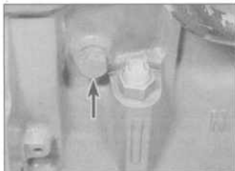
23.18A Oil level sensor location in the cylinder block. Coolant drain plug (arrowed) is adjacent
