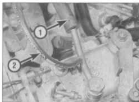
5.9 Main fuel return pipe (1) and injector leak off return pipe (2) (Roto-diesel)
