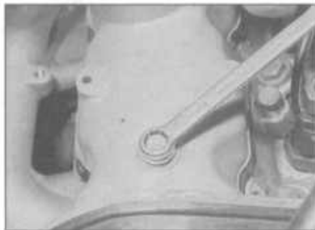
7.8A Unbolt the valve cover ...
