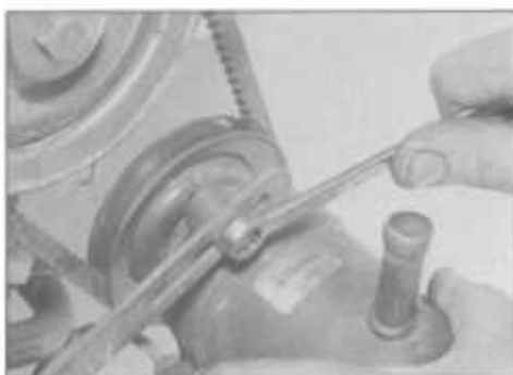
1.2A HP pump adjusting bolt on BX models
