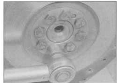
16.6B ... and tighten them to the specified torque
