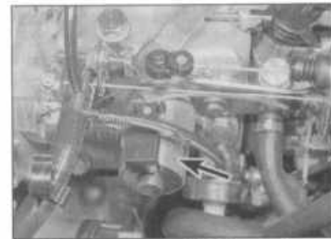
6.3A Electromagnetic timing device (arrowed) - Lucas CAV/Roto-diesel pump
