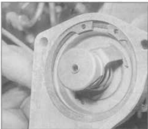
4.4 Thermostat and retaining circlip
