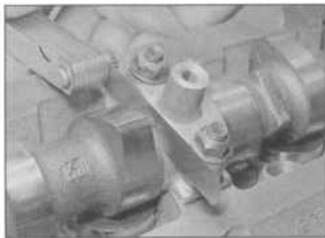
7.20B Checking the camshaft endfloat
