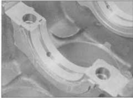
24.3 No 2 main bearing and thrustwashers
