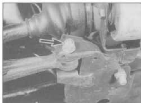
2.2 Front track control arm inner pivot bolt (arrowed) on Visa models
