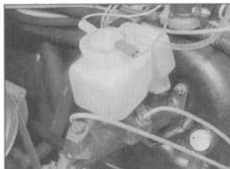
4.1 Brake master cylinder on Visa models
