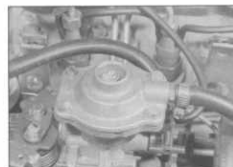
6.5A Richness limiter - Bosch pump
