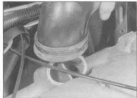
3.4A Disconnecting the air duct from the inlet manifold
