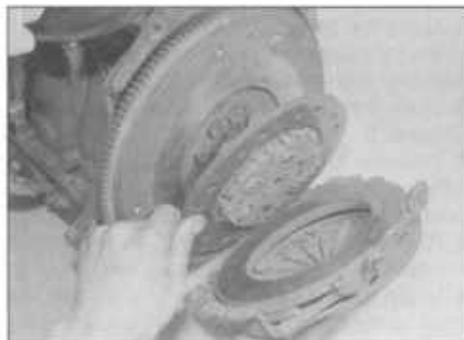
16.2 Removing the clutch pressure plate and driven plate
