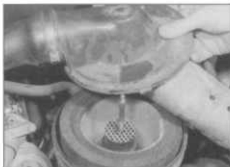
3.7B . . . and lift off the air cleaner cover (BX models)
