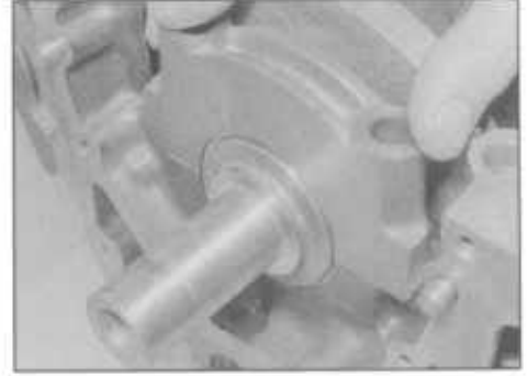
24.8 Fitting No 5 main bearing cap
