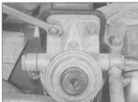
23.3 Removing the Roto-diesel filter head and cartridge
