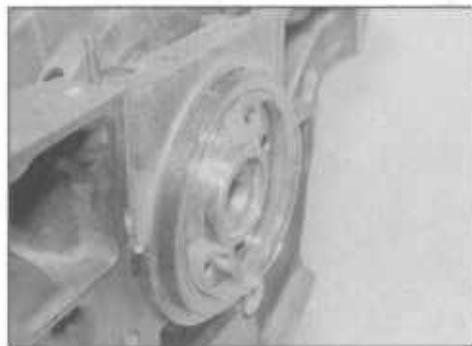
24.14 Fitting the crankshaft rear oil seal with a plastic protector
