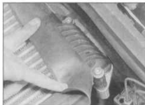
22.3 Pulling back the rubber seal to reveal the rear securing screws
