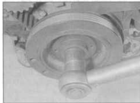
24.62B Tightening the crankshaft pulley bolt
