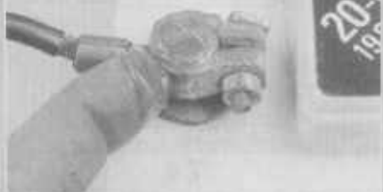
Applying petroleum jelly to the battery clamps
