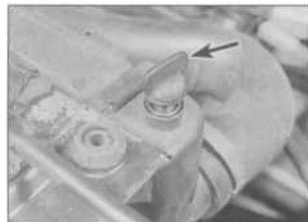
24.14B Bleed screw (arrowed) on the radiator (BX models)
