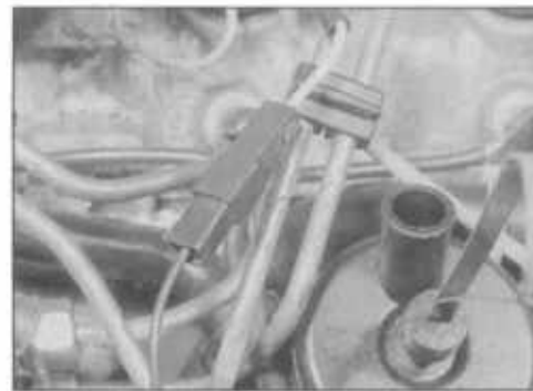
23.3A Diagnostic socket wiring connector
