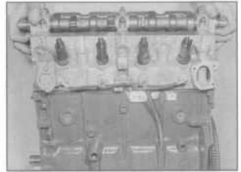
24.38 Lowering the cylinder head onto the block
