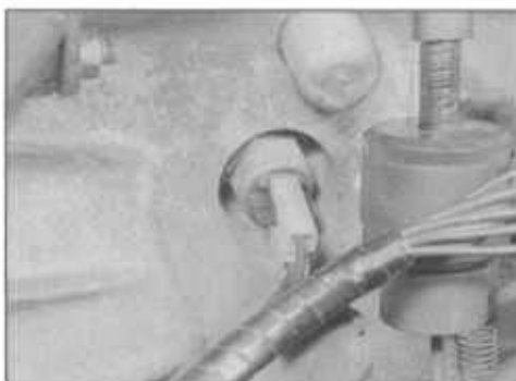
21.3 Reversing lamp switch and wiring
