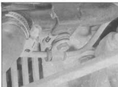
21.7B Hydraulic line and bracket (BX models)
