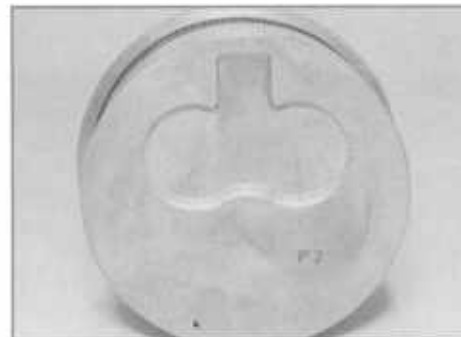
26.25C Clover leaf cut-out on the piston crown
