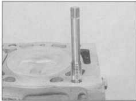
24.34 Cleaning the cylinder head bolt holes with a tap
