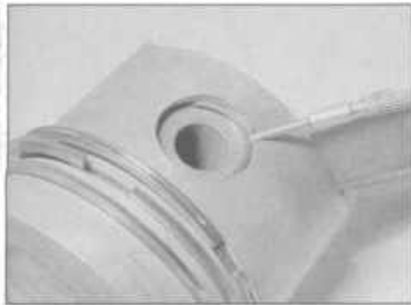
26.22A Prising out the gudgeon pin circlip
