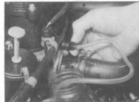
23.9 Draining the fuel from the fuel filter housing
