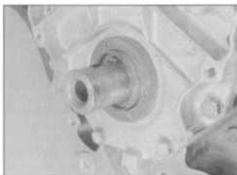
12.26 Fitting the timing belt end oil seal to the crankshaft with a plastic protector
