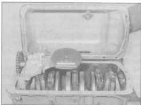
13.6 Removing the sump
