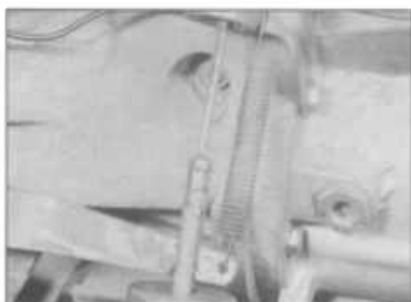
2.8A Clutch cable and lever return spring
