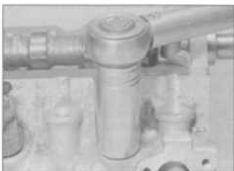
15.15B Tightening an injector
