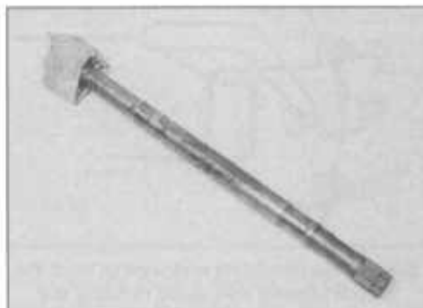
4.8 Left-hand driveshaft with rollers retained with adhesive tape
