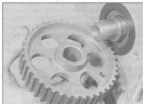
7.9B Removing the camshaft sprocket
