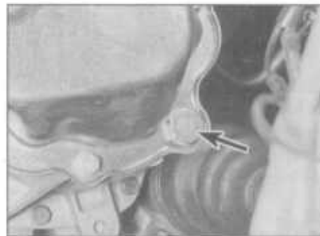
25.6 Manual transmission filler/level plug (arrowed) in end cover
