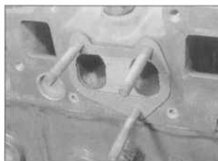
25.7B Exhaust manifold gasket
