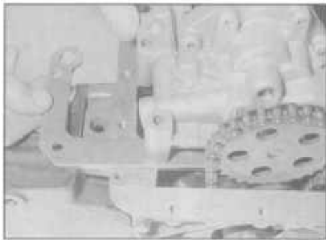
23.46 Withdrawing the oil pump spacer
