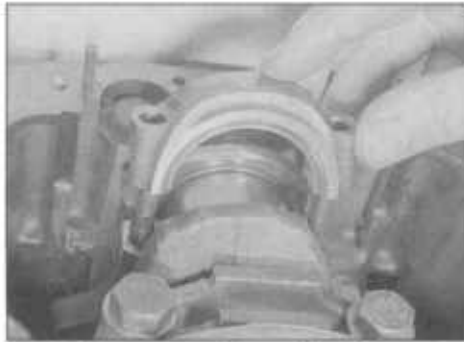
15.5 Removing a big-end bearing cap
