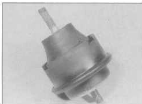
17.2B Engine mounting rubber showing slots
