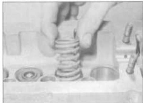
10.6B ... large valve spring ...
