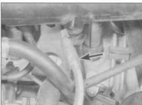
22.4 Disconnecting the hose (arrowed) which runs to the injection pump
