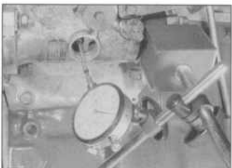
8.13A Timing the Roto-diesel injection pump with a dial test indicator
