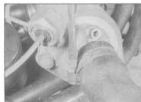
20.16 Disconnecting the top hose from the thermostat housing
