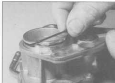
7.3A Removing the large O-ring...
