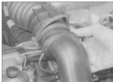
4.1 Unclipping the air intake tube
