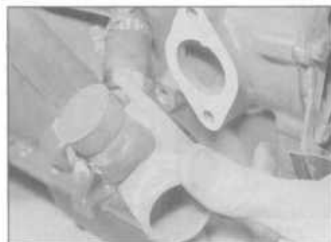
23.21A Removing the water pump inlet
