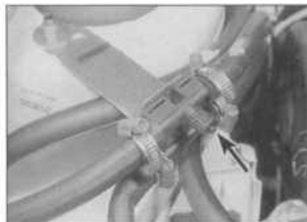
24.14C Bleed screw (arrowed) on the expansion tank return pipe (Visa models)
