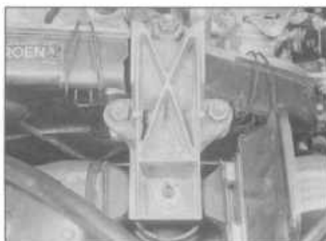
17.3 Right-hand engine mounting bracket (BX models)
