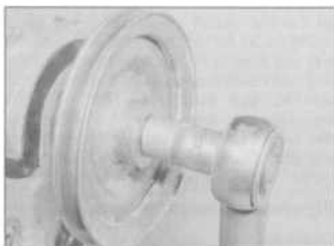
24.81 Tightening the pump pulley bolt on the camshaft
