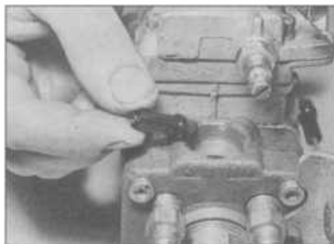
17.5a Removing the stop solenoid plunger from the pump
