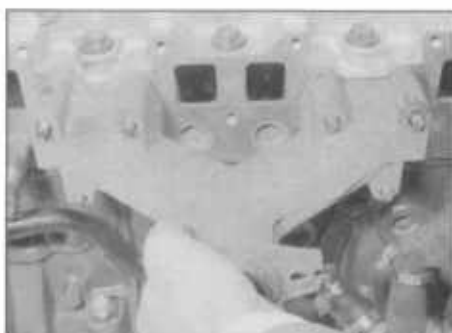
25.7A Removing the exhaust manifold on a 1.9 engine
