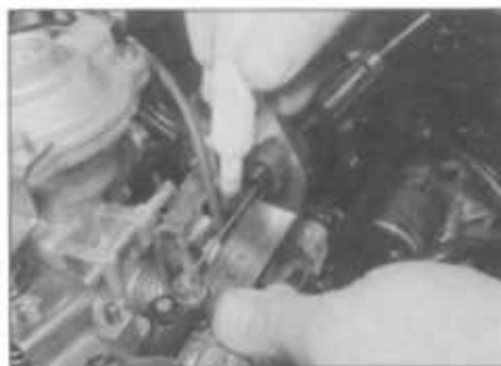
13.1 Marking the accelerator inner cable 11.0 mm from the end of the outer cable
