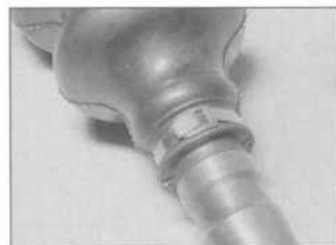
4.15B . . . and bend it back under the buckle
