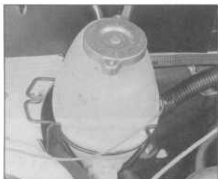
24.2 Expansion tank and filler cap on Visa models
