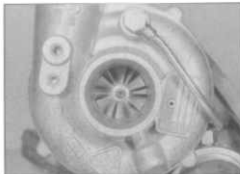
1.11 View of the compressor wheel end of the turbocharger (KKK type)
