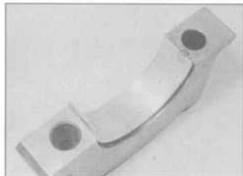
23.56 Main bearing cap and lower half bearing shell
