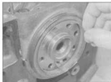
12.33A Fitting the flywheel end oil seal to the crankshaft with a plastic protector
