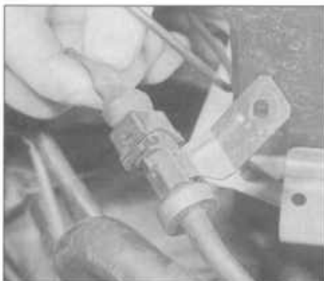
6.2 Removing the turbo over-pressure warning switch
