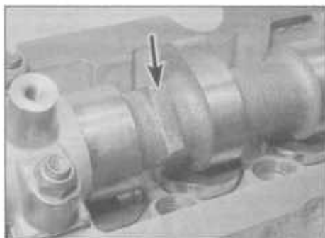
7.9A Special lug (arrowed) for holding the camshaft
