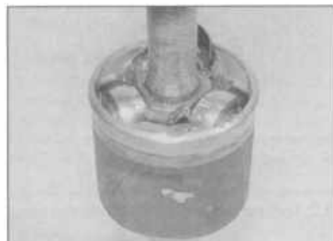
4.7 Separating the driveshaft and rollers from the inner joint housing
