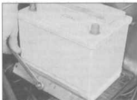
20.15B Removing the battery clamp
