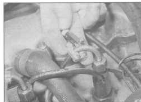
3.14 Clamping a timing light transducer onto an injector pipe
