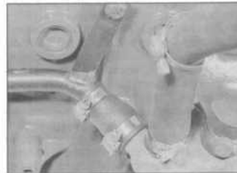
23.21C Coolant tube mounting on the front of the cylinder block
