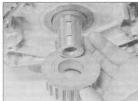
24.46 Fitting the sprocket to the crankshaft
