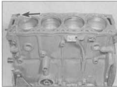
24.35 Head gasket fitted to cylinder block with location dowel arrowed
