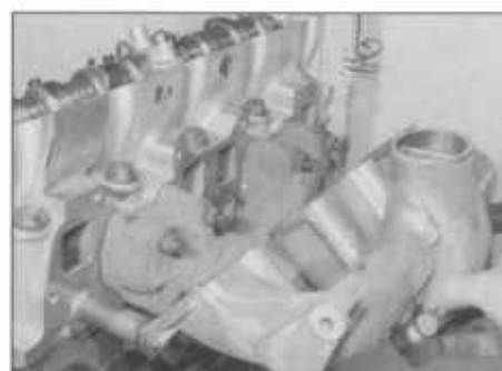
25.3B Removing the inlet manifold (engine removed from car)
