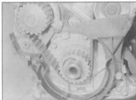
24.60 Bottom timing cover fitted
