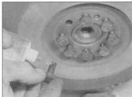
16.6A Apply locking fluid to the flywheel bolts ...
