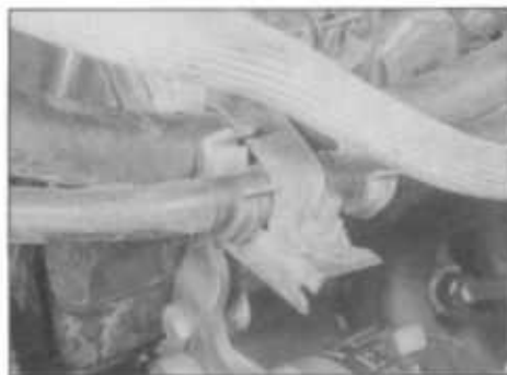
20.26 Hydraulic pipe retaining clip (BX models)
